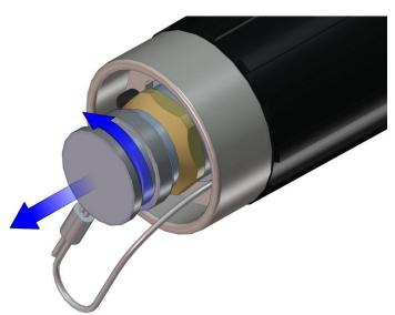
1. To remove the Jaws from the Holmatro 4240 Spreader, you must first relieve all pressure from the system by removing the CORE connection plug from the back of the Spreader unit. Make sure there is no excess oil in the system prior to removing the Jaws.
