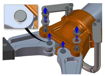
3. Flip the Spreader Assembly over onto its "back" side revealing the Jaw Pivot retaining clips and nuts on the bottom of the Spreader Assembly. Remove the retaining clips using a pair of needle nosed pliers or clip removal tools. Remove the nuts attached to the main pivot pin using a 15mm socket.
