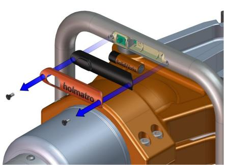
"peel" the gasket off from the handle. It should not rip or tear. Remove the battery from the internal housing and replace as necessary. Make sure to check for excessive corrosion on the battery terminal contacts inside of the handle.
