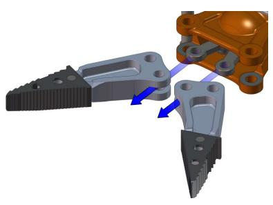
5. The Jaws can now be pulled from the Spreader assembly. Be sure to check the (2) pin holes on both Jaw assemblies as well for excessive wearing or scratches, replacing where necessary. For re-assembly, follow the steps in the reverse order. Apply grease on all (4) of the pins before reinserting into the Spreader Jaws. This will help ensure longevity to your Holmatro 4240 Spreader Assembly.
