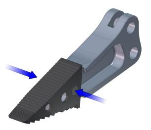
1. The Jaws of the Holmatro 4240 Spreader can be serviced while attached to the Spreader Assembly. However, if extensive service is required, it is recommended to remove them using the proceedures discribed above for removing the Jaws from the Spreader assembly.
